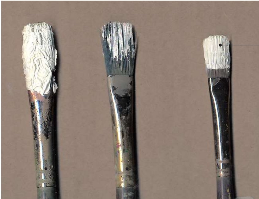
Too much paint
